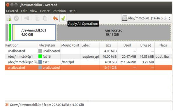
Once the operation is completed. The SDCard can be inserted into Raspberry Pi for image bring up.
