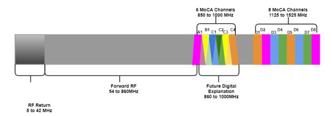
The measure of the MoCA signal, captured in <u>Mbps</u> (PHY Rates), is the baseline measure of MoCA integrity within an X1 home network. Every MoCA device has two paths to every other MoCA device on the same network, one for receiving and one for transmitting. Ideal PHY Rate levels range above 200 Mbps; anything less is considered poor.
