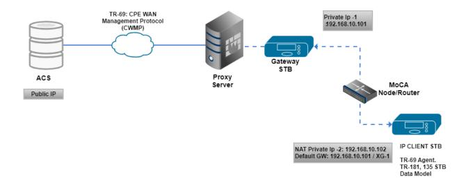
Since the Client is non-addressable from the public network, tr-069 and STUN creates and maintains a lightweight connection between the tr-069 server and agent to allow for tr-069-server initiated commands to be sent to the Client in real-time.
