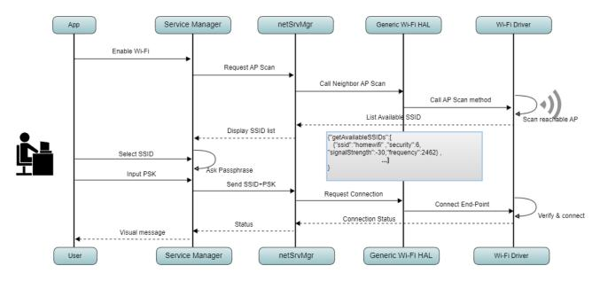
Initiating the connection: Here application may need to enable the WiFi if required. In which case he has call the initialization routine and network manager will handle the further operation
