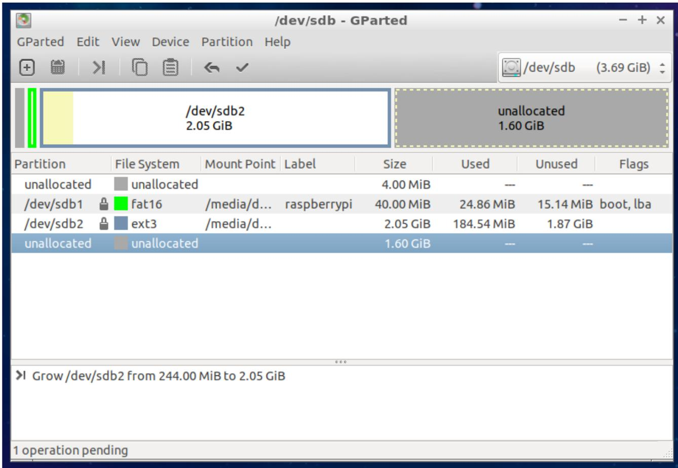
5. After modifying size, "Apply all operations" using tick symbol in UI which displays icon as below
