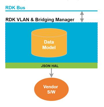
The RDKVLAN&BridgeManagercomponent will hold the Ethernet Link, VLAN Termination, and Bridging data models, and will run processes related to creating or deleting bridges or interfaces
