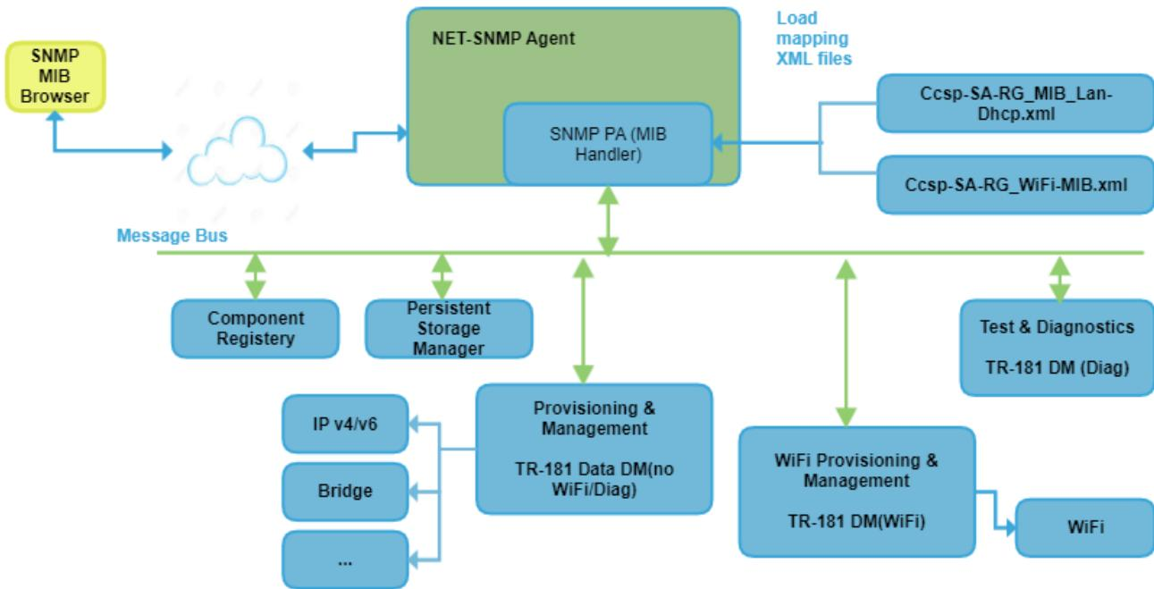
CCSP SNMP Protocol Agent is implemented as a NET-SNMP MIB handler. During startup, it loads all the XML files defining the following:
