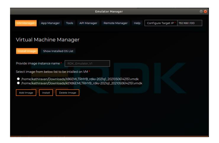
• Show installed OS List: By default, on launch VM manager installed os list will be display (show installed os list tab will be active), developer can see the list of installed images into the vm on the show installed list screen.
