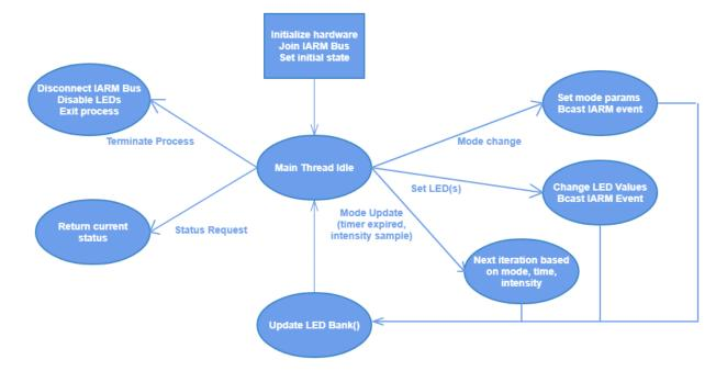
Ledmgr stack contains generic and device specific code. Device specific implementation is in 'extended' folder which has device specific lighting specification. There is a noop implementation provided which can be referred by OEM vendors to implement device specific 'extended' folder.
