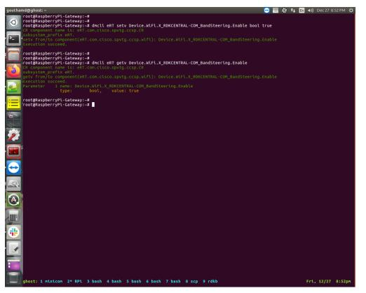
After enabling of Band Steering, the SSID broadcasted by the two interfaces are same. A 5GHz capable client will normally connect to a 5GHz client and older 2.4GHz client will connect to 2.4GHz frequency band.
