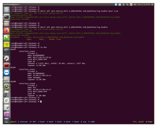
Disabling of Band Steering will reset all previously made configuration on the 5GHz band. Band Steering can be disabled by the below command.
