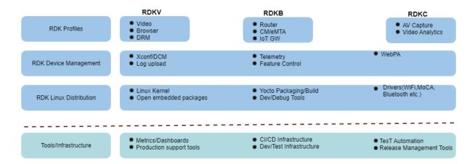
XCONF has client component ie CPE device component and server side component. XCONF's primary purpose is to tell STBs where to send their log files and what telemetry metrics they should be sending. XCONF does not receive logs or telemetry from the boxes. It simply tells the STB where to send log files or telemetry and what specific metrics it should be sending. XCONF also tells STBs when, where (host), and how (protocol) to send this data.
