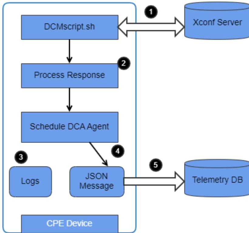
The telemetry upload process is controlled through dcm-log service
