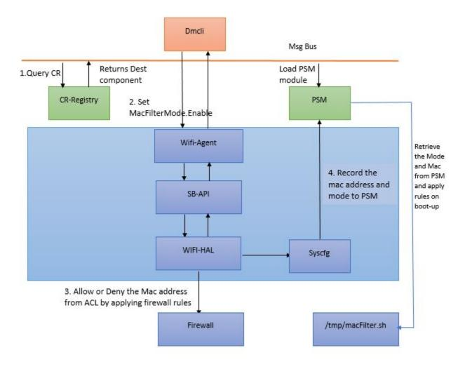
Mac Address are entered via **WEBUI** or **dmcli** and stored in ACL(Access Control List). When the MacFilter mode is set **TRUE**, it involves either white-list or black-list depends on **FilterAsBlackList** value, and applying the iptable rules on mac's in ACL. Also record the FilterMode and mac addresses into PSM (Persistent Storage Manager) by syscfg. Retrieves the FilterMode and Mac on boot-up from PSM, rules are applied by executing the macfilter.sh.
